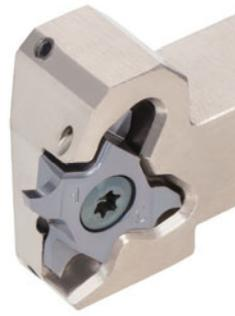
TetraMini-Cut has all of the benefits of the TetraForce-Cut but is smaller insert with same features and offers even greater economy. The insert's width varies from 0.33mm (0.013") to 3.0mm (0.12") with many widths within this range available as a standard, for grooving up to 3.5mm deep, matching or exceeding many three-edged grooving inserts.
