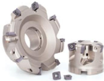
MillQuadFeed allows highly-efficient machining with a large depth of cut up to 2.5 mm and with a high feed rate up to 2.0 mm/t. As the design of insert constraining section and cutting edge prevents lifting of the insert and fracture of cutting edge, a higher stability in machining and fracture resistance have been realized.
