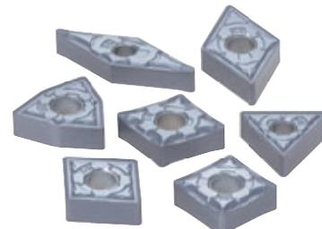
The multi-layered coating with high Al content provided by the new PVD coating technology has ensured strong wear resistance. The new series cover a wider application range in heat-resistant alloy turning from finishing to medium cutting, providing stability and longer tool life.
