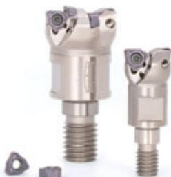
This is a cutter for semi-finishing or finishing operation with profile milling or plunging. By using the double-sided inserts with a positive clearance angle, both the cutting edge strength and the sharpness have been realized. DoMiniMill endures high-feed milling, and the feed speed can be significantly increased by the combination with the multi-flute body.
